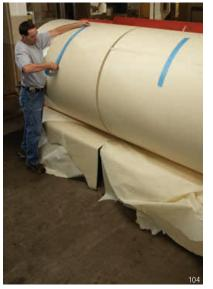
High tack 3M<sup>™</sup> Temporary Single Coated Repulpable Tapes are available in white, blue, and kraft for dependable core starting, roll closing and butt splicing.
