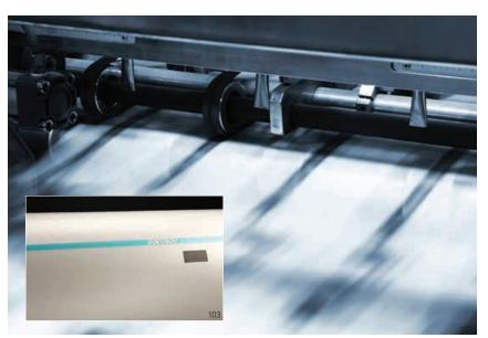
3M<sup>™</sup> Repulpable Splittable Flying Splice Tape eliminates the time and work of "V" and "W" patterns with a straight across flying splice. Advanced coating provides a smooth and consistent opening force. A fiber-free break open means less blanket cleanup.
