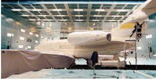
For large and small painting operations, 3M<sup>™</sup> Clean-View Pads protect windows and light fixtures from overspray.
