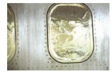
With conformability and chemical resistance, 3M™ Aluminum Foil Tapes protect aircraft windows during harsh chemical paint stripping.
