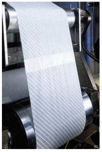
For butt splices on many low surface energy materials such as polyethylene. 3M<sup>™</sup> Super Bond Film Tape 396 provides the thin caliper tensile strength of polyester, and high immediate holding strength of rubber adhesive.
