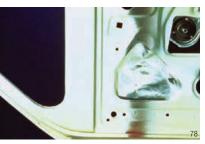
Applied over holes and cavities in the interior of a car or truck door panel,  $3M^{\rm tr}$  Aluminum Foil Tape seals out moisture and dust.
