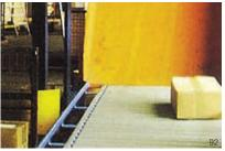
Corrugated boxes slide more easily down a chute lined with abrasion-resistant 3M<sup>™</sup> UHMW-PE Tapes.
