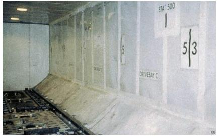
For seaming and sealing panels in aircraft cargo bays, 3M<sup>™</sup> Glass Cloth Tape 398FR exceeds flame retardant standards F.A.R. 25.853 (a) and F.A.R. 25.855 (d). Pressure sensitive acrylic adhesive bonds on contact to many surfaces. High adhesion is secure for extended periods. Rugged cloth surface resists wear from heavy bags.
