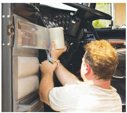
During manufacturing and transport, transparent 3M<sup>™</sup> Polyethylene Protective Tapes protect many finished automotive interior surfaces from abrasion, nicks, and scratches. Clear acrylic adhesive holds with very low tack for easy removal.
