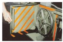
Orange 3M<sup>™</sup> Vinyl Tape identifies dangerous machine parts that may cause injury when enclosure doors are open or guards removed.
