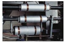
Conformable 3M<sup>™</sup> PTFE Tape helps the movement of web materials in many types of roller wrapping applications.
