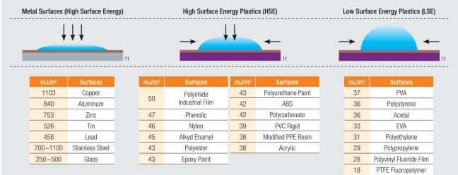
Note: These values are provided as a guide. Formulation modifications can substantially alter surface energies.
