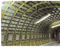
3M<sup>™</sup> Damping Foil 435 between the ribs and stringers of an aircraft fuselage helps reduce vibrational fatigue and noise inside the passenger cabin.
