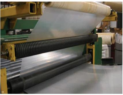
To help ensure a scratch-free surface for the end user, 3M<sup>™</sup> Co-Extruded "A" Tape is applied after final finishing to sinks, spas, and countertops prior to packaging. Enhanced abrasion and puncture resistance protects the surface through shipping and installation. Tape then removes cleanly.
