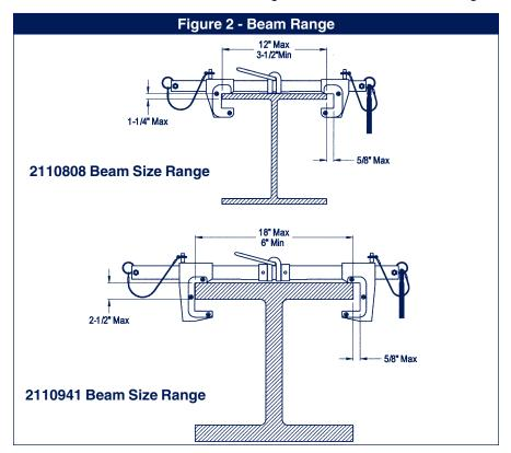
beam anchor is for use as a component of a personal fall arrest system (PFAS). Do not hang, lift, or support tools, equipment, or materials from the sliding beam anchor. Do not use a sliding beam anchor as a lifting point when moving structural members.
