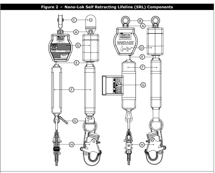
${\bf A}$  - Swivel  ${\bf B}$  -Swivel Eye  ${\bf C}$  - Integral Connector  ${\bf D}$  - Housing  ${\bf E}$  - Web Lifeline  ${\bf F}$  - Load Indicator  ${\bf G}$  - iSafe<sup>TM</sup> RFID Tag  ${\bf H}$  - Snap Hook
