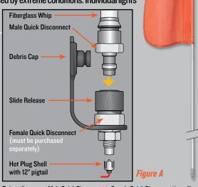
To install, connect Male Quick Disconnect to Female Quick Disconnect by pulling the spring-loaded Slide Release down while firmly pushing the male and female components together and releasing the Slide Release. Attach Hot Plug Shell to the base of the Female Quick Disconnect to supply power to the Whip Light.
