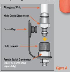
To install, connect Male Quick Disconnect to Female Quick Disconnect by pulling the spring-loaded Slide Release down while firmly pushing the male and female components together and releasing the Slide Release.
