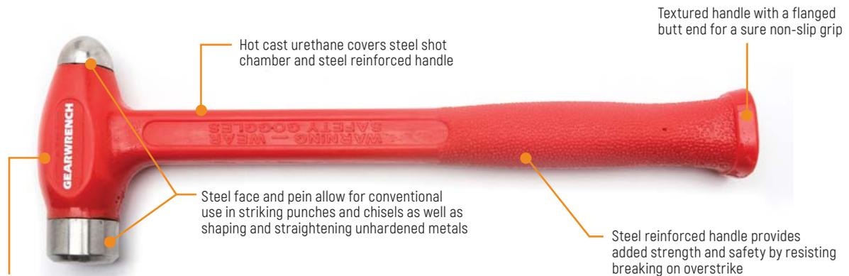
Steel shot filled canister creates a dead blow effect; sustains impact, maximizes force, reduces/eliminates rebound, and absorbs the shock of impact
