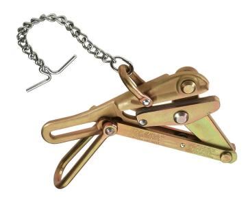
Designed for use on aluminum, copper, weatherproof coated wire, PVC covered conductors and messenger and guy strand. The Chicago style grip was designed for cable sizes from 0.12-Inch to 1.0-Inch (3.10 to 25.4 mm). Equipped with chain, toggle and shackle. For support wire 0.134-Inch and larger, refer to 1659 series. Outside diameter of support wire includes thickness of polyethylene coating.
