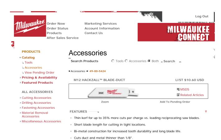
Designed to maximize the cutting performance of the new M12 HACKZALL™ Reciprocating Saw, these blades feature a thin kerf design that reduces the amount of drag and resistance while cutting, resulting in more cuts per battery charge. Specialized blades are available for a variety of HVAC, electrical, plumbing and maintenance/repair applications. Includes 5 blades.
