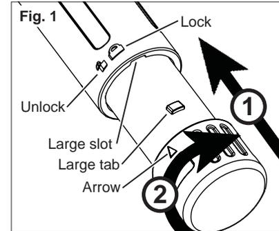
Line up the the large and small tabs on the battery with the large and small slots in the tool opening. Slide the battery all the way into the tool. Turn the battery clockwise to lock it in place. The arrow on the battery will line up with the on the tool.
