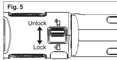
When the battery is installed, the tool is in operating condition. The lock switch prevents accidental starting by locking the forward/reverse switch. Always set the lock switch to "lock" before performing maintenance, changing accessories, storing the tool and any time the tool is not in use.
