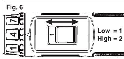
1. For **low** speed (200 RPM) and more torque, push the speed selector back ("1" is displayed).
