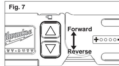
Press and hold the forward/reverse switch up for forward rotation, and down for reverse rotation. The switch will automatically return to the center, OFF position when it is released.
