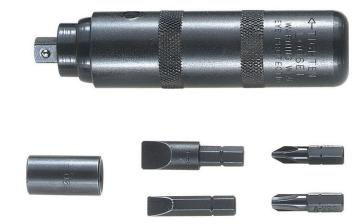
Klein Tools' Reversible Impact-Driver Set is a rugged, hand-impact driver designed to turn rusted, frozen, or other stubborn screws. The internal, spring-loaded, helical design transforms the impact of a hammer blow up to 200 ft. - lbs. of shock torque. It can also be used with 3/8-Inch square-drive impact sockets.
