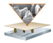
Conventional ceramic abrasive grain tends to "plow" through the metal, causing heat to build up in the workpiece and the abrasive — resulting in a slower cut and shorter abrasive life.
