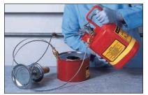
Grounding with antistatic wires
