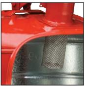
Stainless Steel flame arrester stops flashback ignition, provides faster liquid flow, and offers superior chemical and corrosion resistance. Long 3-1/2" (88mm) length for safe, secure insertion of gas nozzle
