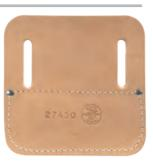
**Connecting Bar Holder** with Lock Collar Lock Collar fits Klein<sup>®</sup> 7/8" (22 mm) connecting Bars (Cat. Nos. 3246 & 3248). Leather construction. Tunnel loop allows for weight distribution on belt. Fits belts up to 3-1/2" (89 mm) wide. Replacement lock collar
