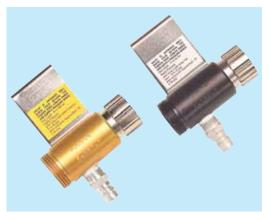
High-pressure control valve is designed to deliver the required air flow to the facepiece at an inlet pressure range of 35-40 psig for hose lengths of 8 to 300 feet. Low-pressure control valve is designed to deliver the required air flow to the facepiece at an inlet pressure range of 10-15 psig for hose lengths of 8 to 50 feet. The valve includes an integral belt clip and male and female quick-disconnect assemblies. (See back page for parts information chart).
