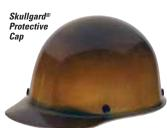
Skullgard Caps and Hats feature heavy-duty construction for use in steel mills and other heavy industries where elevated temperatures are common. Skullgard Caps and Hats meet or exceed the applicable requirements for a Type I helmet (top impact) as outlined in ANSI Z89.1-2003, Class G (electricallow voltage).
