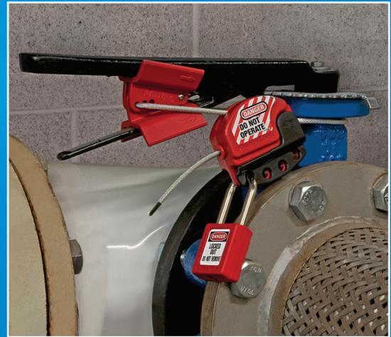
S806 with Butterfly Valve secured with 410RED
