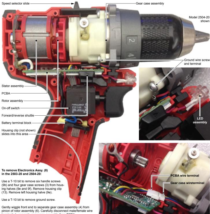
terminals to separate gear case assembly from PCBA.
