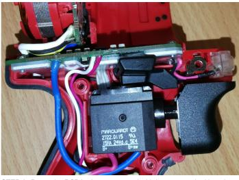
**STEP 8:** Route the PCBA wires connected with battery terminal into the wire channel of left housing as shown.
