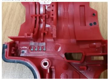
STEP 1: Insert light pipe in cavity of left housing halve-support.
