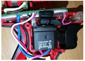
**STEP 7:** Install forward/reverse shuttle and on-off switch into left housing halve-support. Be sure shuttle is properly seated over the forward/reverse tab on top of on-off switch.
