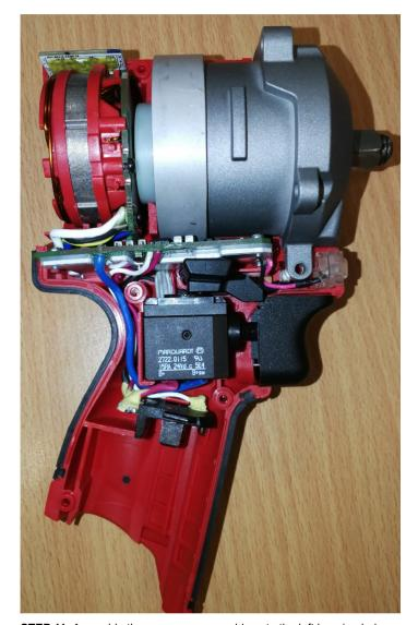
**STEP 11:** Assemble the gear case assembly onto the left housing halve and secure with two gear case screws.
