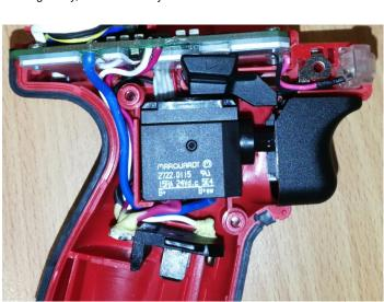
**STEP 10:** Install battery terminal block into the housing halve being sure that it is firmly and squarely seated in the cavity.
