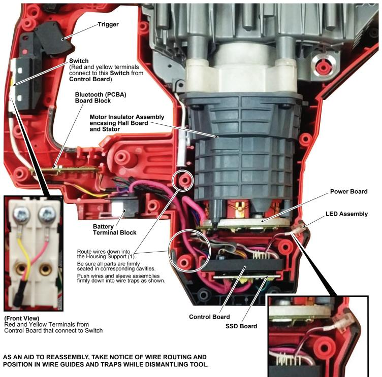
BE SURE THAT ALL COMPONENTS OF THE ELECTRONICS KIT ARE SEATED FIRMLY AND SQUARELY IN THE HANDLE RECESSES.
