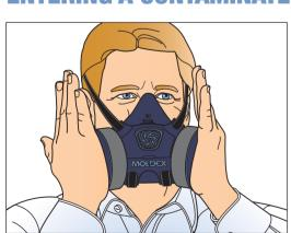
**Negative Pressure Seal Check: Cover** both cartridges without pressing too hard against face, and gently inhale and hold your breath. The facepiece should slightly collapse. If air leakage is detected, re-adjust the position of the facepiece and the tension of both headstraps and repeat the seal check until leakage is eliminated.
