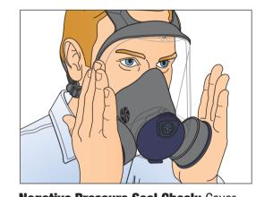
**Negative Pressure Seal Check: Cover** both cartridges without pressing too hard against face, then gently inhale and hold your breath. The facepiece should slightly collapse. If air leakage is detected, re-adjust the position of the facepiece and the tension of head harness and repeat the seal check until leakage is eliminated.
