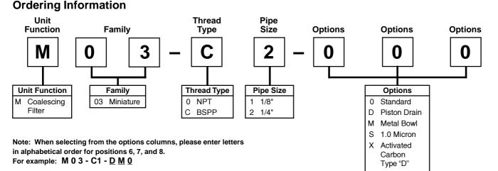
NOTE: 000 in position 6, 7, and 8 signifies standard product. (Poly Bowl, Manual Drain, .01 Micron "C" Element)
