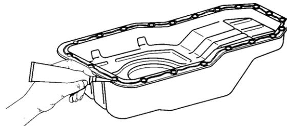
6. Assemble parts immediately while silicone is still wet.
