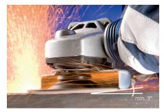
Very low grinding angles create a large surface contact area and very comfortable grinding position.
