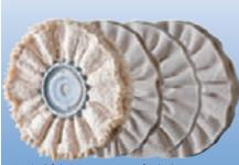
ST sisal fabric TW soft cloth TH hard cloth FL flannel These cloth rings are available in four types: ST sisal fabric = pre-polishing TH hard cloth = pre-polishing TW soft cloth = high-gloss polishing FL flannel = high-gloss polishing Cloth rings used with polishing pastes for prepolishing and high-gloss polishing tasks. For very smooth finishes it may be recommended to use several, or even all, types in succession.
