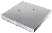
**Aluminum Cylinder Base** – For use when an enlarged cylinder base is needed or advantageous. Attaches to bottom of RA556, RA556L and RA5510 with four  $\frac{3}{8}$ ”-16 screws (included). Serrated base for extra stability.
