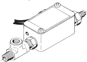
The #9625 Pressure Switch can be mounted directly to a control valve manifold or can be mounted in-line. The switch is designed to stop the pump motor or electrical device at a pressure setting and to restart the motor when pressure falls below that setting.
