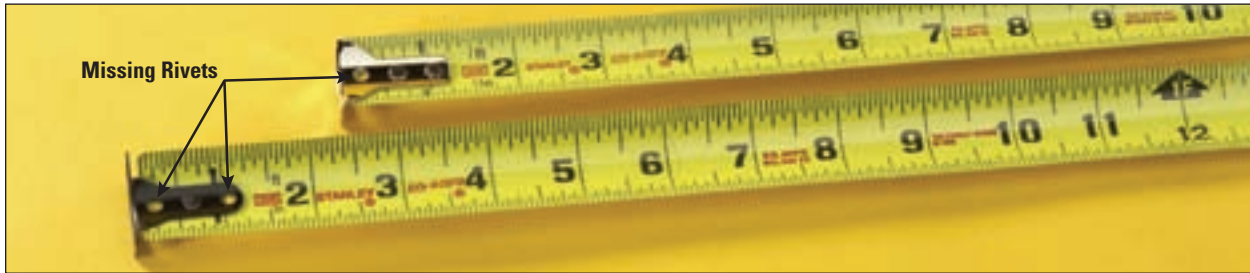
Missing Hook Rivets
