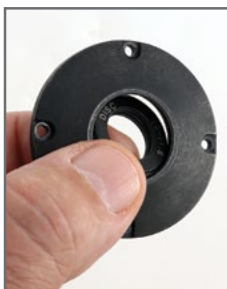
Insert Black Gold coolant ring into cap
