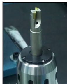
Coolant-thru tool installed
