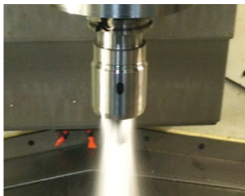
Coolant is channeled directly onto tool path.
