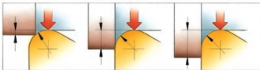
The relationship between nose radius and DOC affects vibration tendencies. It is often an advantage to choose a nose radius which is smaller than the D O C.
