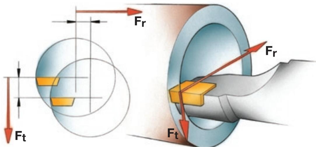
Radial and tangential cutting forces deflect the boring bar during machining, often necessitating cutting edge compensation and tool damping.
