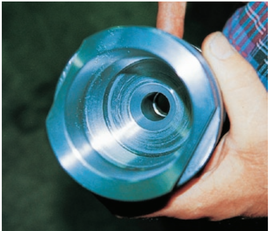
Off-centre drill usually produces incorrect hole sizes.
