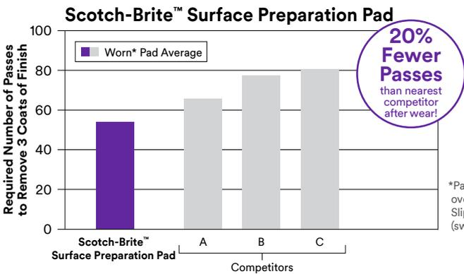
\*Pads worn via 25 passes over 3M™ Safety-Walk™ Slip-Resistant Treads 610 (swing machine)
