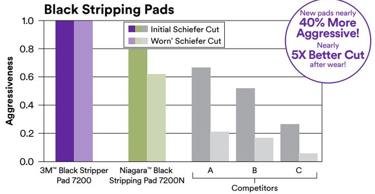
\*Pads worn via 50 passes over 3M™ Safety-Walk™ Slip-Resistant Treads 610 (swing machine)
