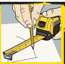
**TIP 7** Use the conveniently diamond marked 40 cm/16" centres for setting out joists.
