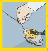
**STEP 5** Rewind away from the marked line to avoid contaminating the work surface and line.
