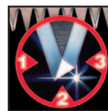
SHARPTOOTH™ TECHNOLOGY UTILIZES THREE CUTTING SURFACES.
