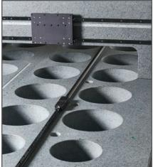
Using precision equipment in our assembly laboratories, we can provide you with the next level assembly, such as adding bearing rails, encoder rails, screw drives, stages, or vibration damping devices.
