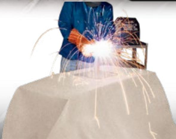
Welding blankets and rolls are widely used for draping over equipment or floor surfaces in welding areas, or as a vertical shield to protect from sparks, spatter, and slag.
