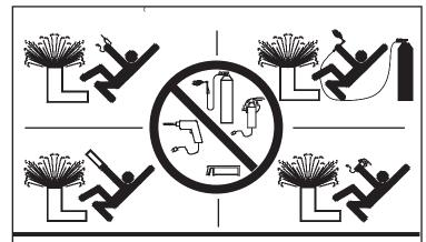
Danger of explosion. Do not drill, grind, saw, weld or use a torch on this product. Doing so could result in serious injury, death or property damage.
