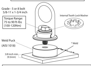
\* Welding procedure must be approved by an engineer or other qualified person to be compatible with any and all structural & operational characteristics of the selected installation location.
