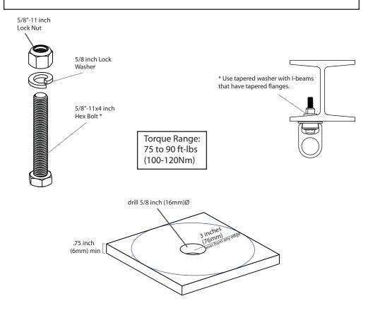
\* For steel applications at grade-5, an 8 (or equivalent) bolt no shorter than 4 inches (100mm) with a locking nut and washer must be used. Swivel anchor must be flush with steel surface. A 16mm bolt may be used in place of a 5/8-11 inch for metric applications.
