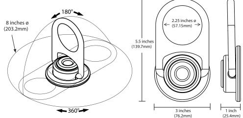
Minimum Breaking Strength (MBS): 10,000-lbf (44kN)
