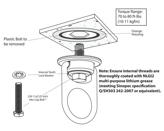
WARNING: Do not install if insert was knocked over during installation. Mega Swivel must mount flush to surface when fastened with the proper torque.
