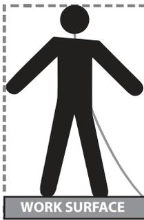
\*The user shall be equipped with a means of limiting the maximum dynamic forces exerted on the user during the arrest of a fall to a maximum of 1800-lbf (8 kN).
