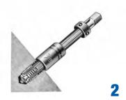
Push the holder down until it touches the broken tap. Slide the sleeve down until it touches the work. (Both are important.)
