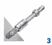
Apply a tap wrench to the square end of the holder. Twist forward and backward a few times to loosen, then back out the broken tap.
