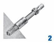
Push the holder down until it touches the broken tap. Slide the sleeve down until it touches the work. (Both are important.)
