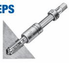
Thoroughly remove all chips of the broken tap. Insert the extractor fingers into the flutes of the broken tap, pushing them gently but firmly into position.
