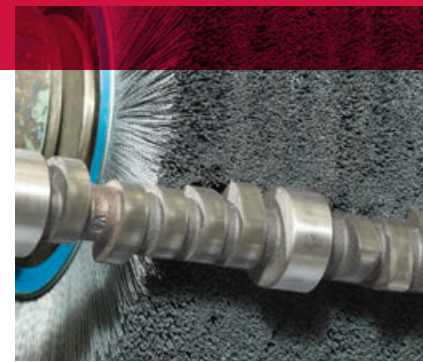
Deburring a camshaft with a Nylox wheel.
