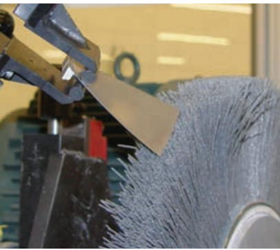
Deburring the tip of a turbine blade.
