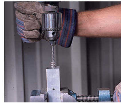
Crosshole deburring an aluminum manifold.
